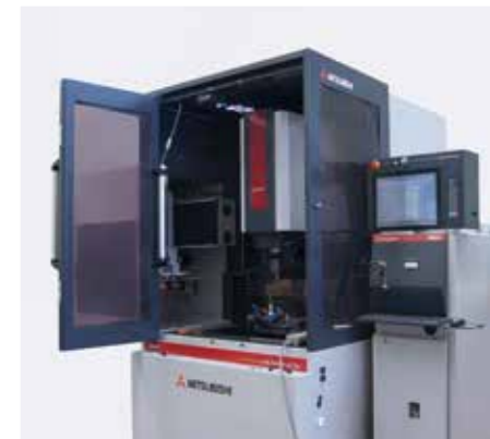
Sistmolding’s toolshop is notable for its EDM section with numerous wire-cutting and die-sinking machines from Mitsubishi Electric.
