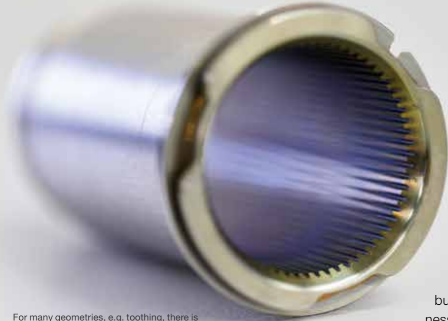
For many geometries, e.g. toothing, there is no alternative to wire-cutting
