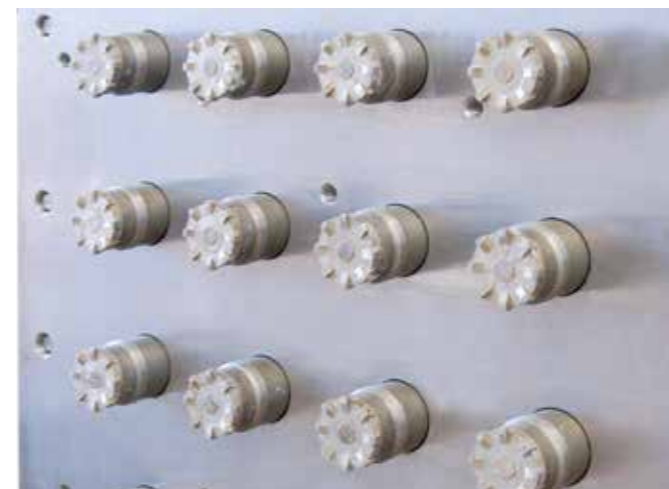
The hot-runner injector invented by Sistmolding to eliminate costly and bulky sprues.
