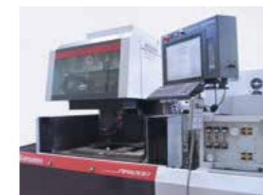
Sistmolding’s toolshop is notable for its EDM section with numerous wire-cutting and die-sinking machines from Mitsubishi Electric.
